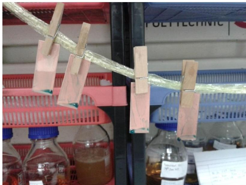
Figure 3.11.1: Copper samples drying
